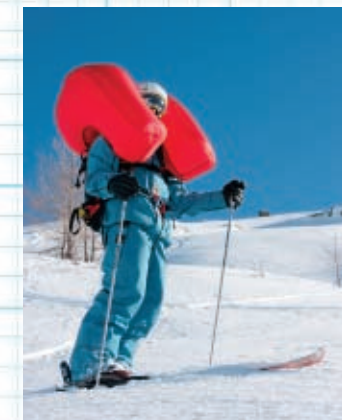
The backcountry industry has seen a recent spike in new inflatable avalanche flotation devices. Top: The new Avi Vest in field testing. Bottom: A diagram showing how the Snowpulse avalanche airbag prevents burial.
